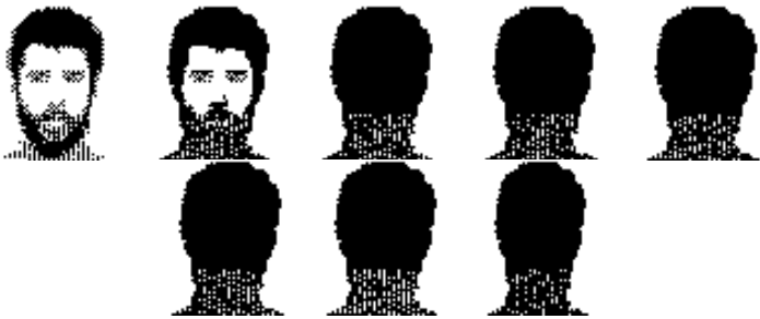
Fig. 29. These are the consecutive bit-planes from most significant to least significant.
