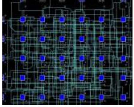
Fig. 2. Marked layout of PREP benchmark #4 with a 96-bit mark
